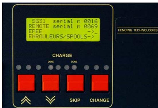
The first line can't be modified. It just gives the unique address of the machine. This unique address will identify the machine unequivocally when the machine is connected to the integrated LAN.
