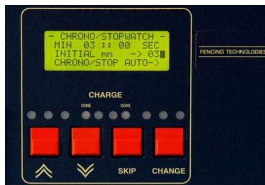
This screen is devoted to the stopwatch. The second line displays the current state of the stopwatch. It is not updated in real time during a bout in order not to slow the machine down. What's more, this is not necessary as the stopwatch is also displayed directly on the machine.
