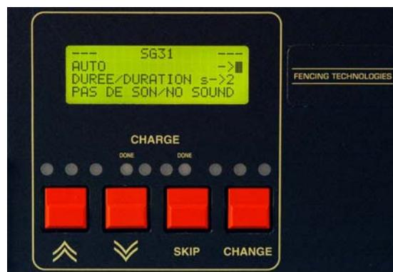
The second line allows for selection of AUTOMATIC or MANUAL mode.
