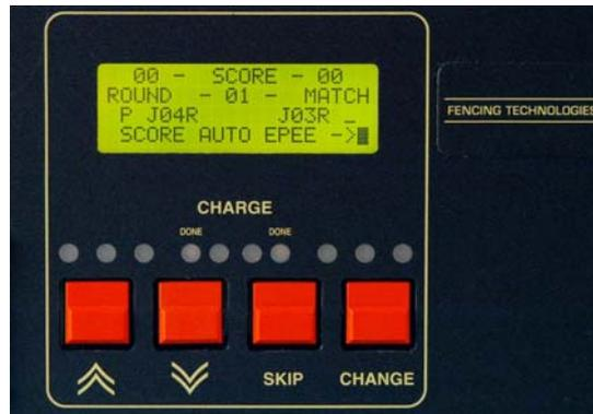
This first line displays the current SCORE and is updated in real time. The score itself is controlled through the remote control (for more information, consult the section devoted to the remote control) or directly on the front panel. Turning the score ON or OFF can only be accomplished through this last method.
