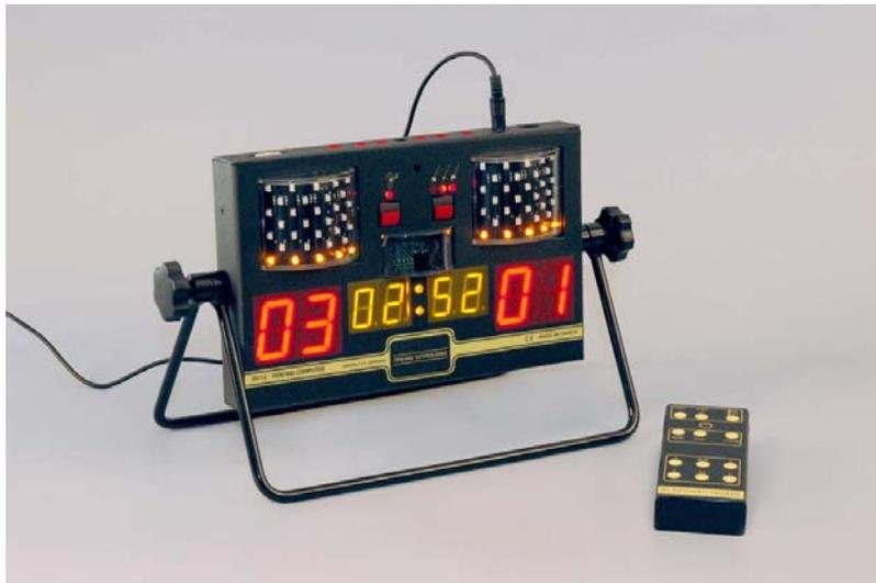
The lights used to indicate a short between the fencer's vest and his weapon in the foil and saber (antifraud lights) are located on the top line of the matrix.
