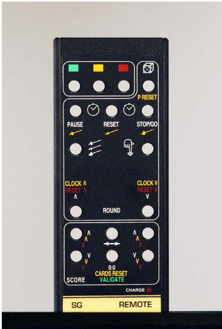
**Each button on the remote control may have up to three different functions.** The main function is indicated by a white text or drawing, the second function is in yellow while the third (if there is one) is in red.
